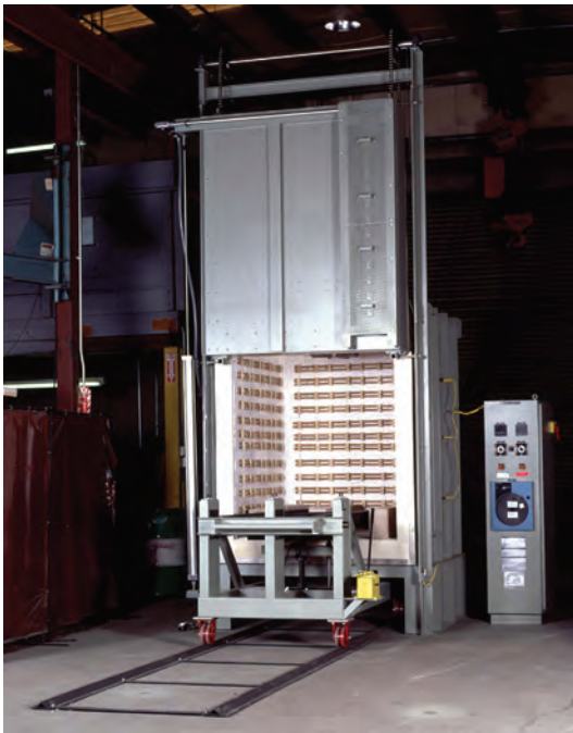
This Model FB 454 features a pneumatically operated vertical door with a NEMA 12 control panel and a 2000 pound hydraulic loader.
