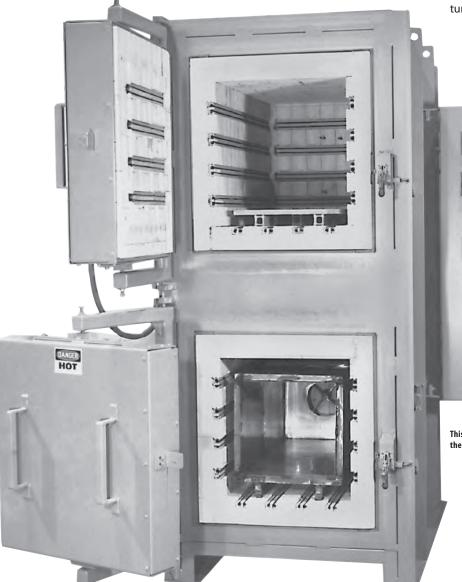
This is actually a photograph of a regular QD furnace. On the QDH, the fan and recirculation muffle is on the top.
